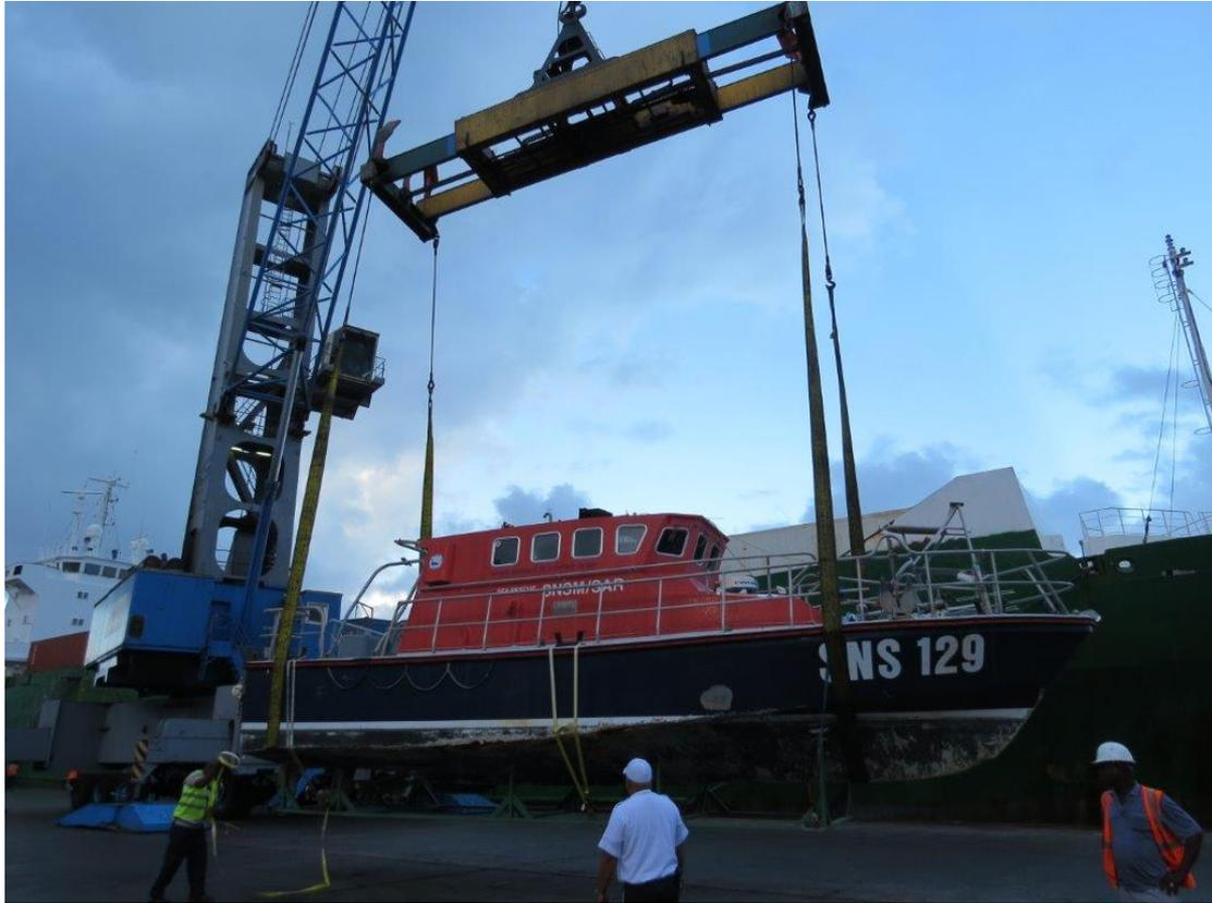
**PHOTO CUTLINE:** CEO SNS129 being loaded onboard CMA CGM Midas MV by a Port St. Maarten Mobile Gottwald Crane in preparation for its journey to Guadeloupe earlier this week.
